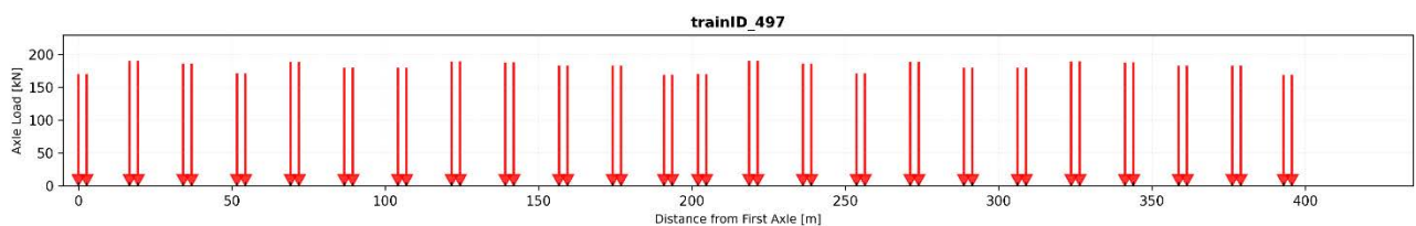
Figure 68. Axle spacing and load of a real ABa train that induce vibrations in bridges that are not covered by the reference DTC2 ABa train in some cases.
