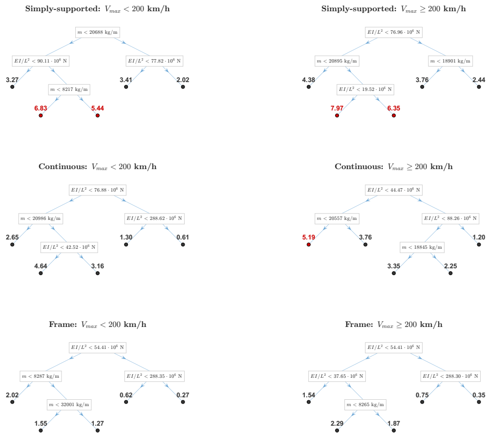
Figure 46: Regression tree for the multi-parametric prediction of vertical bridge acceleration. The terminal nodes show the mean predicted acceleration in \text{m/s}^2 . A color saturation is applied to acceleration values \geq 5 \text{ m/s}^2 .
